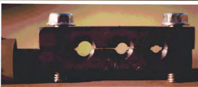
Figure 5: Low cost swaging tools can be purchased which utilize the compression of two bolts to compress cable sleeves. This particular model is designed to squeeze three popular American size sleeves. Note the poor indexing between the two tool halves. This results in an unevenly compressed cable fitting. While strength tests have not been performed on completed cable ends, the results do not generate confidence. There are better quality tools on the market, which are used by airplane mechanics to make cable repairs within confined spaces.
