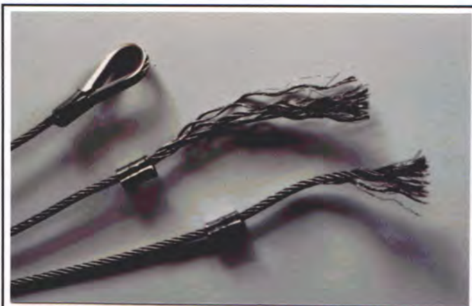
Figure 3: This photo shows the frayed ends of two cables which slipped from their swaged sleeves. The failures are attributed to improper compression of the sleeves. These cables had been in service for several years.
